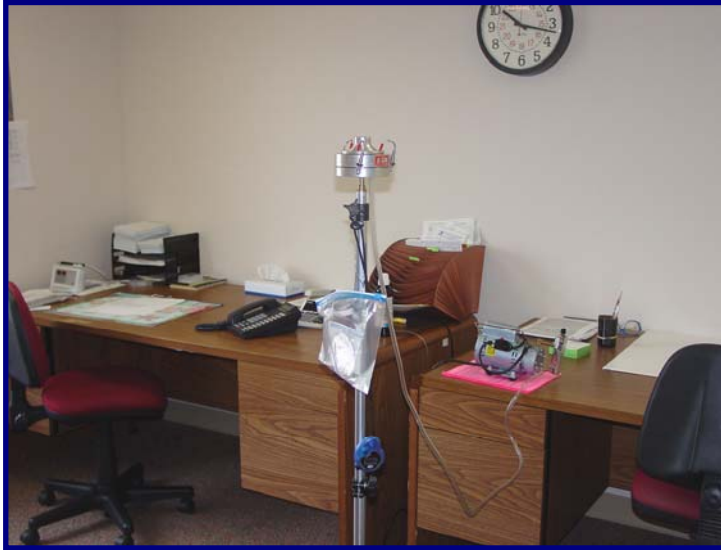
Figure 1. Single-stage multi-orifice viable air sampler (Andersen N-6).
